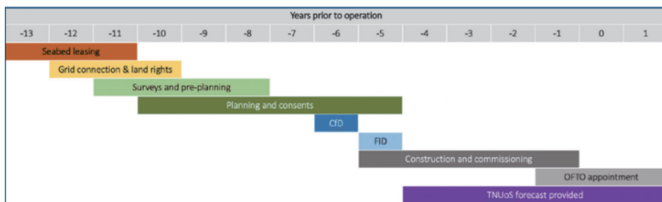
From OTNR presentation, December 2020 Figure 6 Lead time for the development and construction of an offshore windfarm
